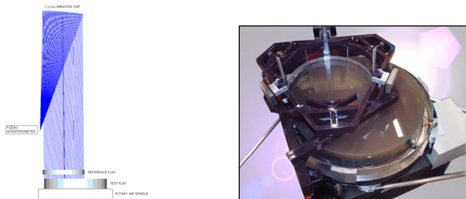
Figure 5A: Test Setup for measuring multiple apertures of a larger optic. On the left, the diagram shows the beam propagating from the interferometer (far left) to an off axis parabola (top left), then down to the transmission flat and test flat. In the right image, the top optic is the calibrated 1.0 meter transmission flat and bottom optic is the 1.6 meter test flat. The remote Fizeau cavity is the gap between these two flats. Courtesy of College of Optical Sciences (University of Arizona).
